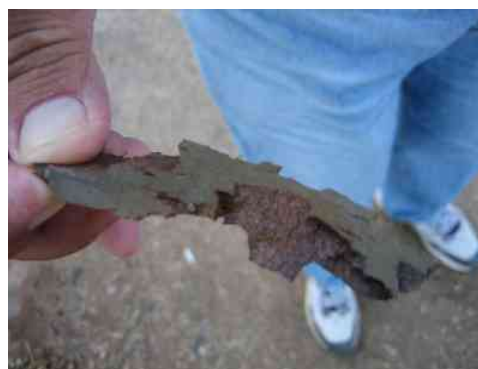
Right: Steel shrapnel showing sharp, brittle fractures.
